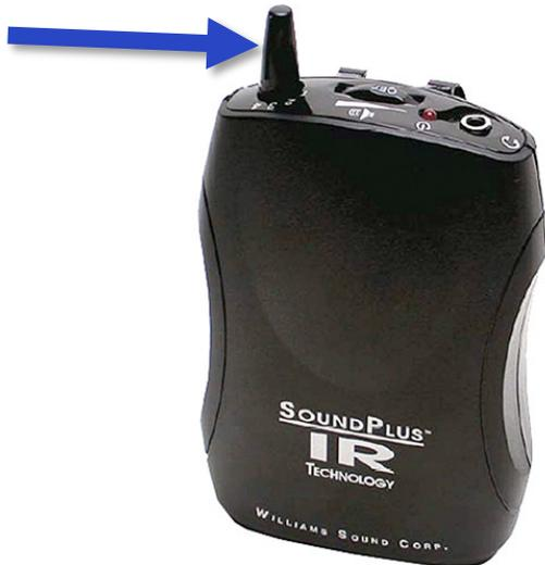
**Step 2** – You can turn on and adjust the volume of the headset using this dial:
