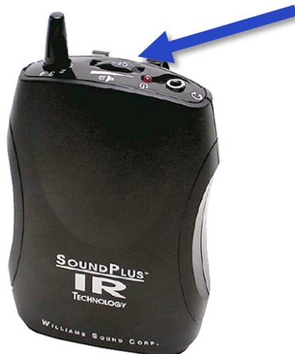
**Step 3** – Using the strap on the receiver pack, wear the pack around your neck with the pack resting on your chest. Make sure there is no clothing or other obstacles covering the receiver pack: if the pack is covered, it will be unable to receive the infrared signal from the transmitter in the room, causing the sound quality of the headset to diminish or disappear entirely.
